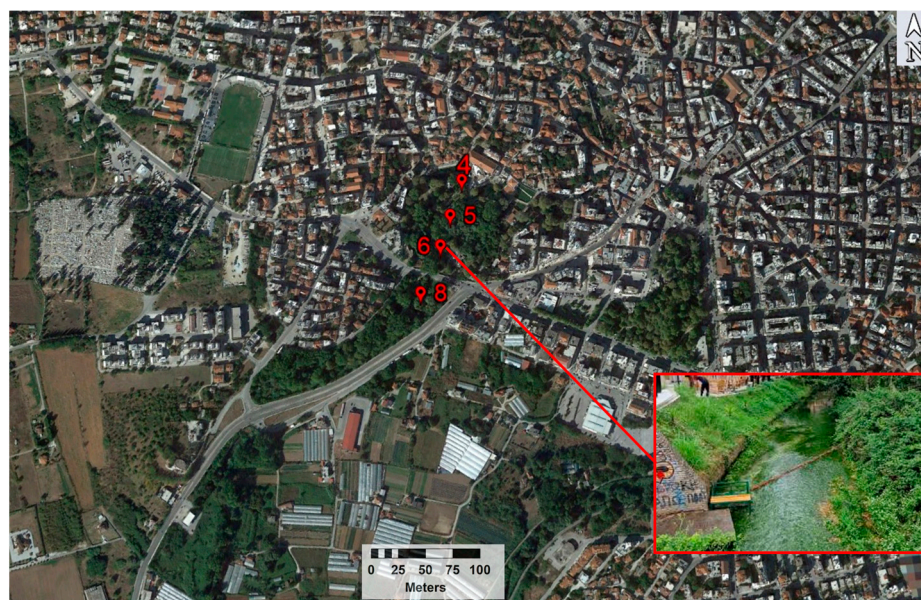
Figure 13. The five opportunity sites for the installation of the litter trap in Agia Varvara Park. Cross-sections 5 and 6 were optimal. The litter trap was installed in cross-section 6, as can be seen in the inset photo.
