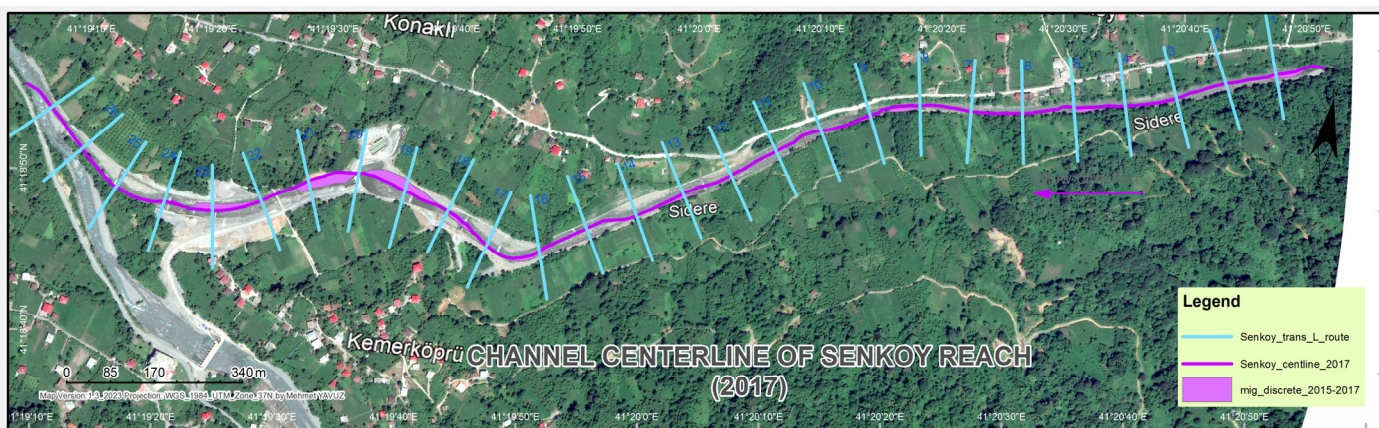
Figure 2. The stream channel centerline (magenta) and cross-section lines (blue) that were used for channel migration analysis from 2015 to 2017 for the Senkoy Village Reach site within the Arhavi River Watershed (Türkiye).
