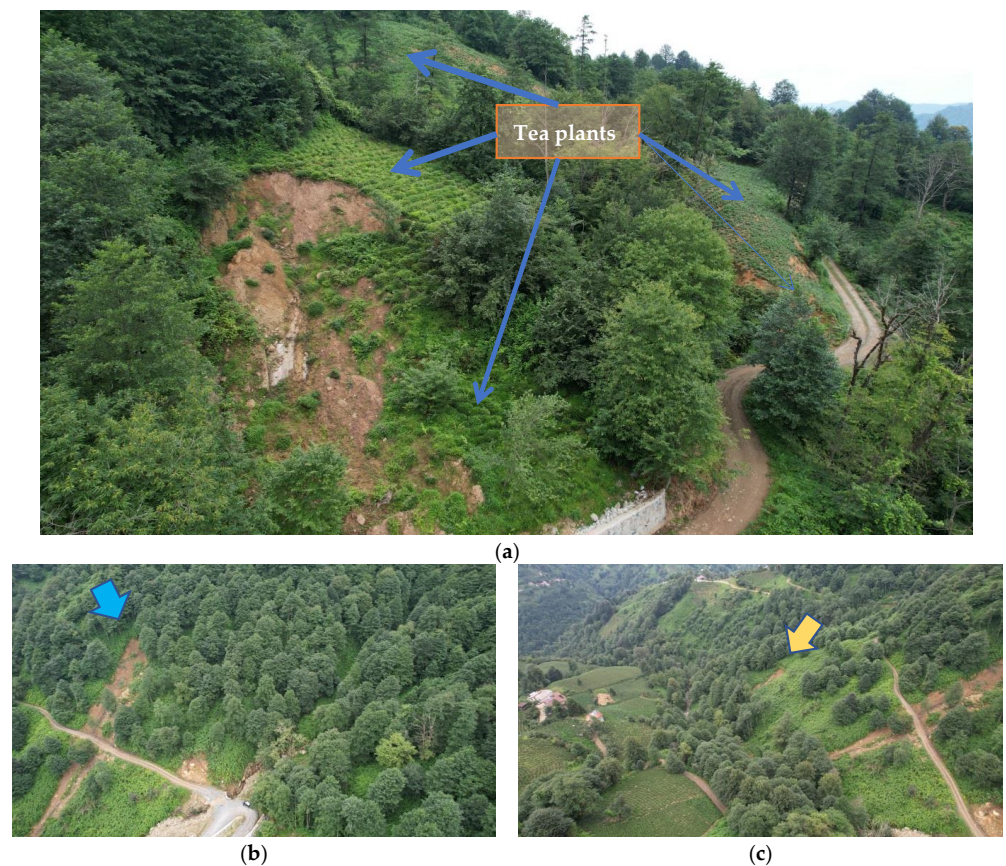
Figure 17. The landslides were triggered by a heavy rainfall event on 22 July 2021 in Sirtoba, Arhavi, Turkey: (a) a translational landslide within a tea garden near Sirtoba; (b) a debris avalanche (blue arrow) within a forest in near Sirtoba that affected the road network; (c) a relatively small translational shallow landslide (yellow arrow) within a pasture near Sirtoba.
