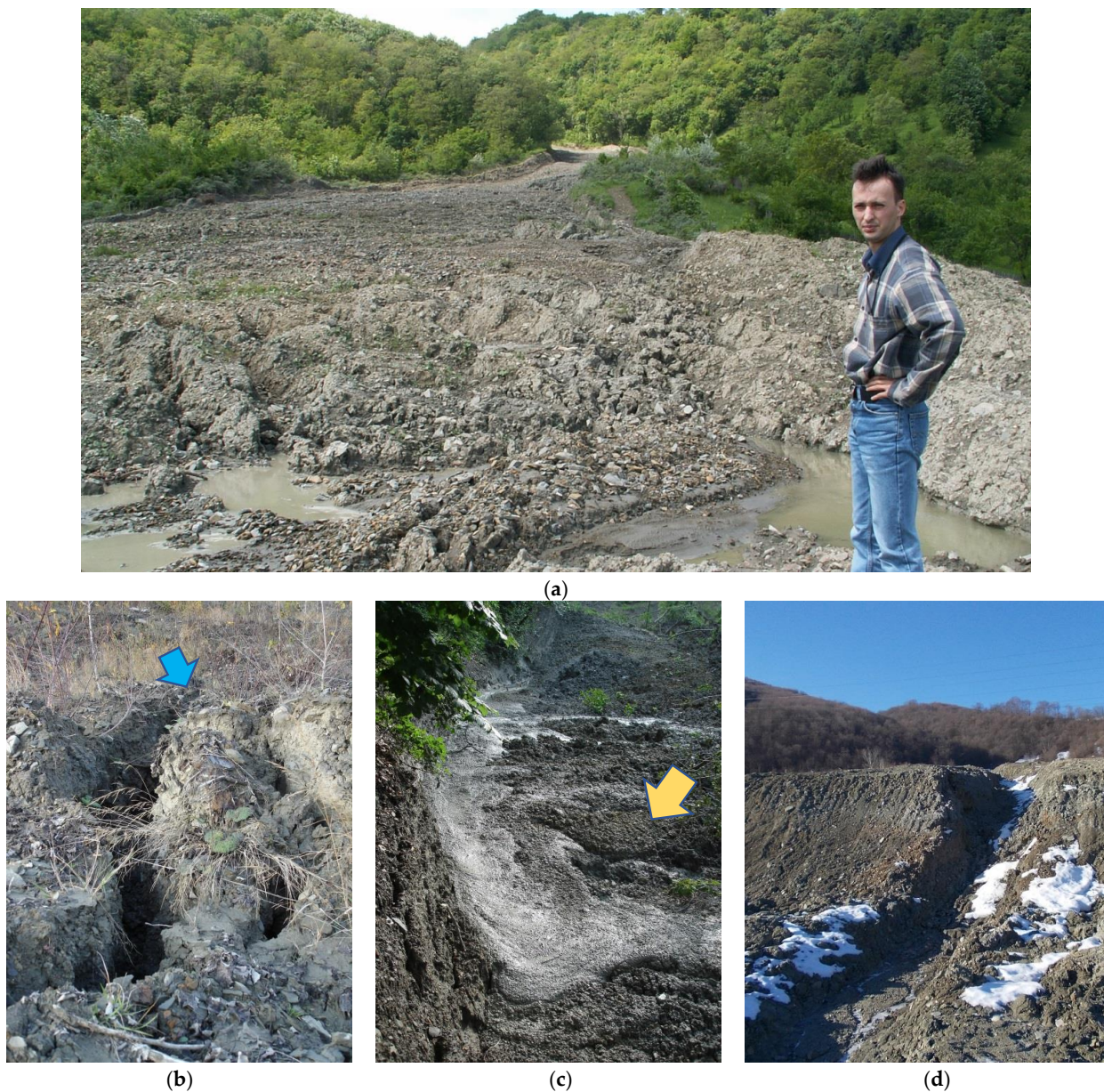
Figure 18. The Chirlesti mudflow site in Romania: (a) Daniel C. Diaconu standing on mudflow debris that was deposited on a nearly flat surface, and the road below was threatened near Chirlesti; (b) ruptures (blue arrow) along right and left flanks of the affected area; (c) a mudflow phenomenon (yellow arrow) is still in progress; and (d) a recent photo of the study area showing the height of mudflow debris from Chirlesti Village Road (photos by Daniel C. Diaconu).
