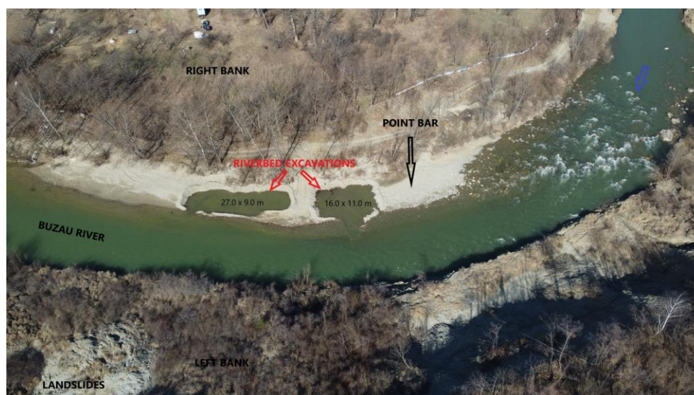
Figure 8. The aerial image of the excavated river bed from the DJI Mavic Mini 2 drone taken at 100 m height.
