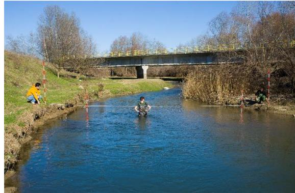
**Figure 1. a. Erosion Pins installed on stream banks. b. Stream Cross-sections measurements**
