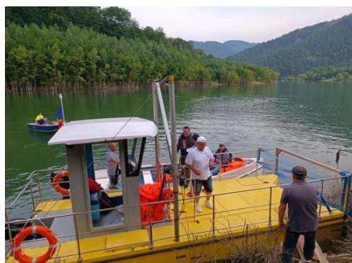
Photo 3. Skimmer vessel with deck installed
