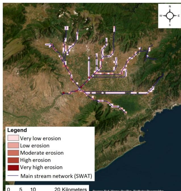
**Figure 3.** The GIS Stream Bank Erosion Index for the Aggitis Basin in the main SWAT's stream network. Five classes represent different rates of stream bank erosion: very low, low, moderate, high and very high.
