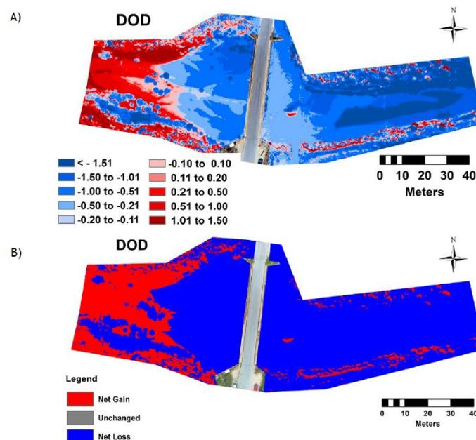
**Figure 2.** The DoD resulted from the comparison of the images between the dates 14 September 2022 (a) and 28 October 2022 (b). The colorized scale represents the different elevation categories (in meters). The 3 classes: (red) gained material, (grey) unchanged elevation and (blue) loss material.
