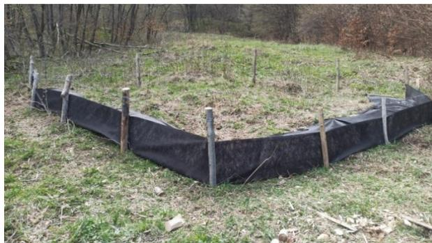
Fig.1. Sketch of a type alluvial Gerlach trap
