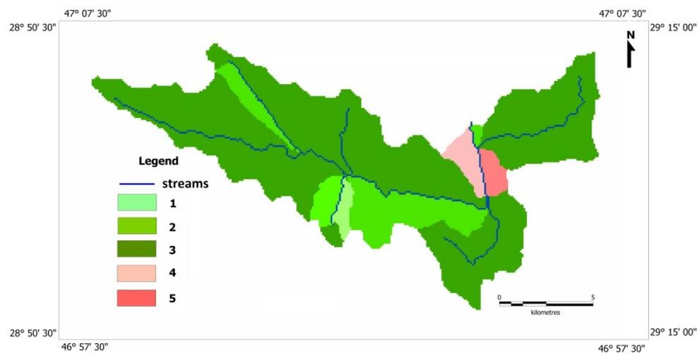
**Figure 3.** Map of GeoWEPP offsite simulation of annual sediments distribution in the Baltata River watershed for the period 1990-2010. The sediment yield (ton) is classified as: 1)  $0 \leq \text{Yield} < \frac{1}{4}$ ; 2)  $\frac{1}{4} \leq \text{Yield} < \frac{1}{2}$ ; 3)  $\frac{1}{2} \leq \text{Yield} < 1$ ; 4)  $1.0 \leq \text{Yield} < 2.0$ ; 5)  $2.0 \leq \text{Yield} < 3.0$ .
