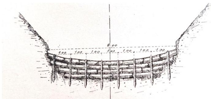
**Figure 3.** Wooden check dam on torrents in French (Source: Thierry [8])
