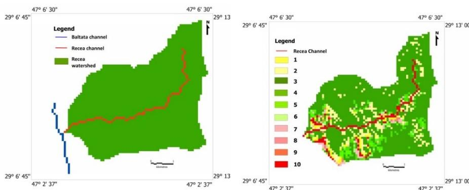
**Figure 2.** a) the offsite and b) onsite simulation of annual soil loss and sediment deposition in the Recea watershed for 1990-2010. The sediment deposition and soil loss (ton) is classified as: 1)  $< 1.0$ ; 2)  $< 1.0$ ; 3)  $0 \leq \text{Loss} < 1.4$ ; 4)  $1/4 \leq \text{Loss} < 1/2$ , 5)  $1/2 \leq \text{Loss} < 3/4$ ; 6)  $3/4 \leq \text{Loss} < 1$ ; 7)  $1.0 \leq \text{Loss} < 2.0$ ; 8)  $2.0 \leq \text{Loss} < 3.0$ , 9)  $3.0 \leq \text{Loss} < 4.0$  and 10)  $> 4$  ton
