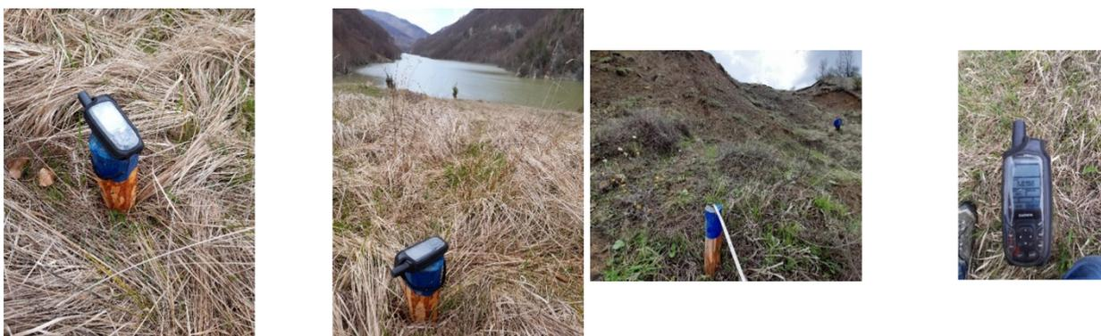
Fig.3. The pins installed to determine the current mobility of the Wind Pit landslide from the Siriu reservoir and the Păltineni landslide - the left slope of the Buzau River
