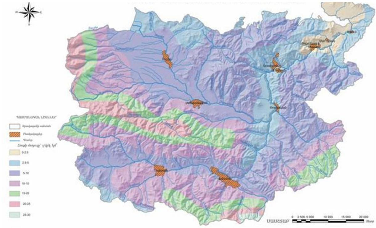
Figure 3.15. Flow module of Debed River Basin
